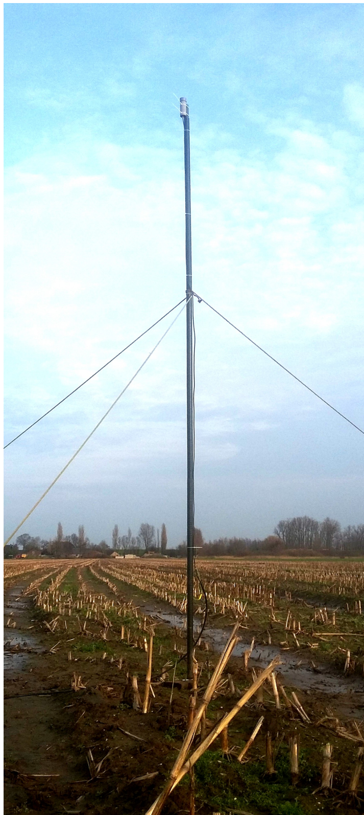
The Mini-Whip on a 350cm pole in the field.
