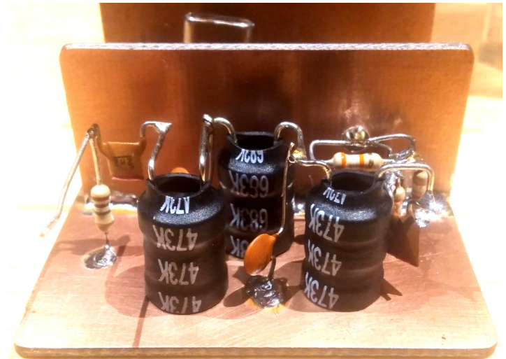
The input filter with 47 and 68 mH inductors.
