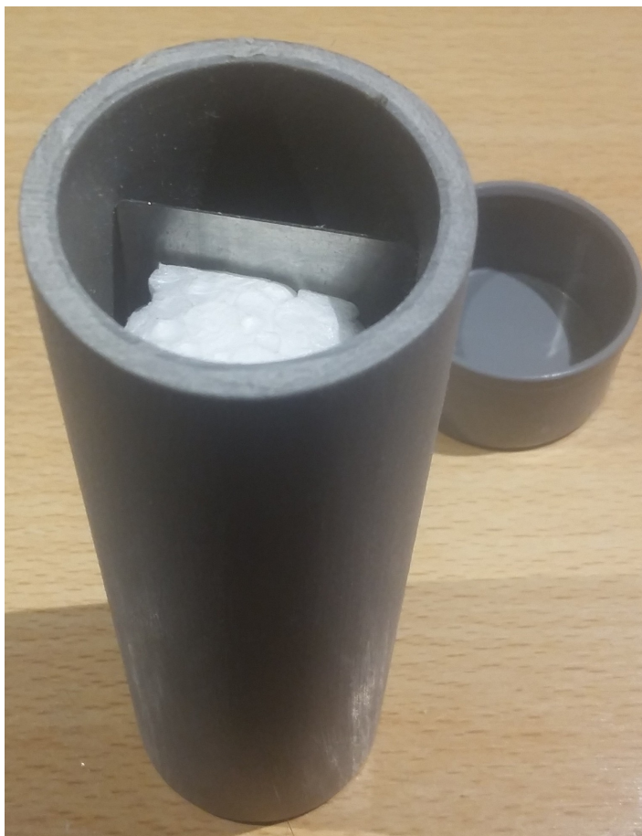
I put the PCB and probe in a piece of drain pipe, using some foam to keep it in place.
