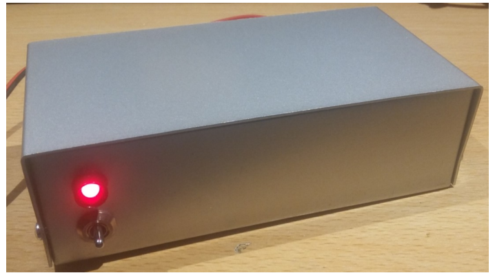
The final result: a nice box with power switch and LED indicator. Connectors for 12Vdc, RF in and RF out are on the back.
