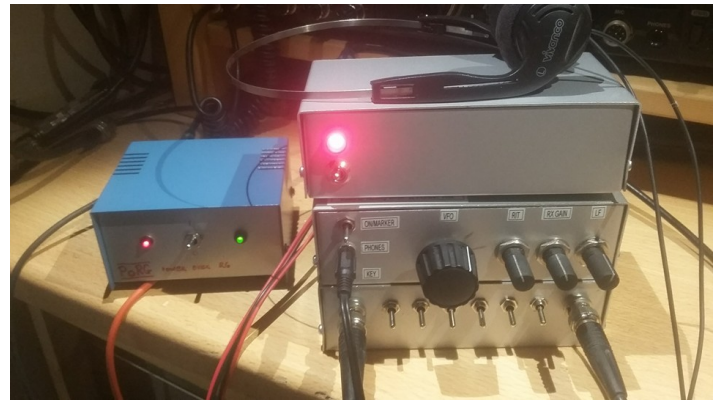
PoRG (left), VLF-converter (on top), 30m transceiver (middle) and step attenuator (bottom).
